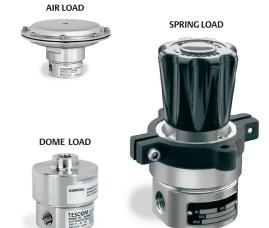
TESCOM 26-2300 Series is a highly accurate, diaphragm sensed backpressure regulator. It controls pressures up to 500 psig / 34.5 bar and offers many C<sub>V</sub>s from 0.02 up to 1.0. Air and dome loaded versions are available for remote operation or for use with the TESCOM ER5000 Electropneumatic Controller for automation.
